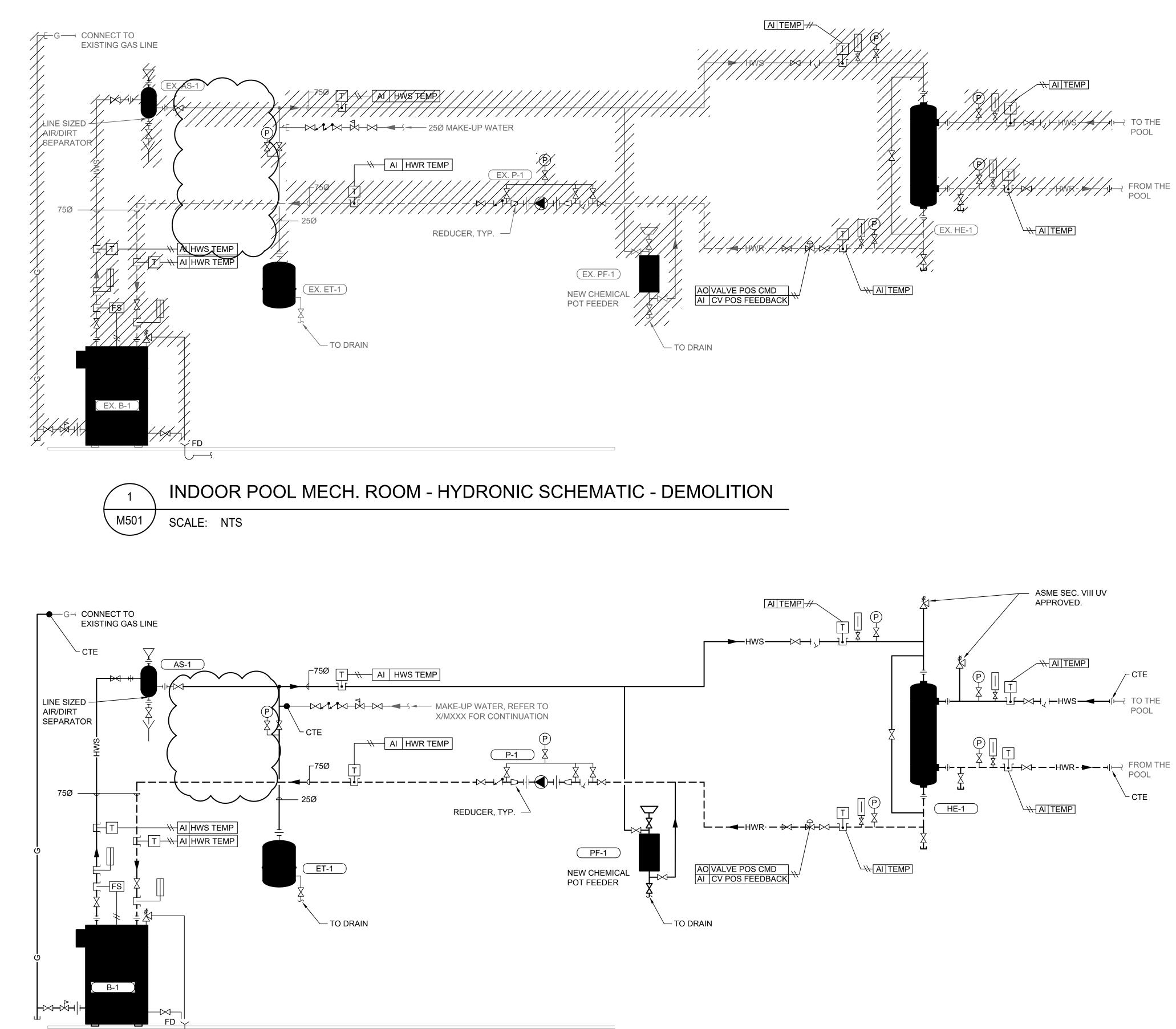
INDOOR POOL MECH. ROOM - HYDRONIC SCHEMATIC - RENOVATION 2 M501 SCALE: NTS
